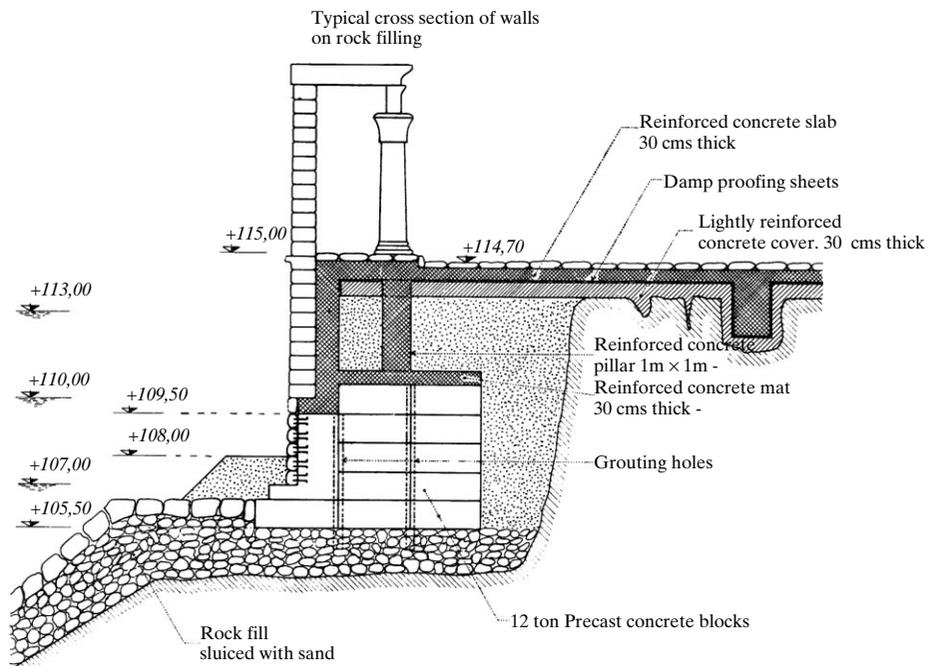
Fig. 5: Cross section for the proposed foundation of the new temple
